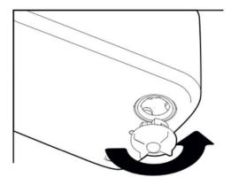
Remove the drain plug by turning in the arrow direction.
